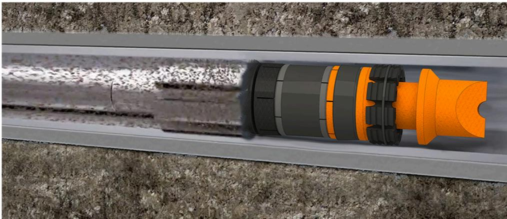
Quality built non-aggressive reverse style bladed junk mills offer the best performance if a mill is preferred or if there is a high sand environment. The non-aggressive style helps to minimize motor stalls and keep cuttings consistent. PDC bits also work very well in all applications.
